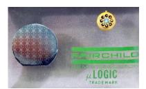
With just seven parts, Fairchild announced the world's first standard logic family of integrated circuits, direct-coupled-transistor-logic (DCTL), in March 1961 based on Hoerni and Last's resistor-resistor-transistor (RTL) planar process under the  $\mu$ Logic trademark. One of these devices, the  $\mu$ L903 3-input NOR gate, became the basic building block of the Apollo guidance computer. Designed by MIT and built by Raytheon, it needed 5,000 devices
