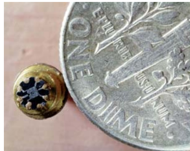
First Prototype Planar IC integrating four transistors and six resistors – May 1960
