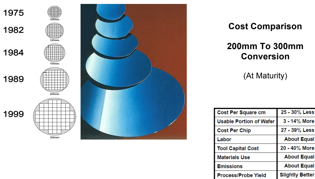
Figure 9 – Previous Wafer Size Transitions
